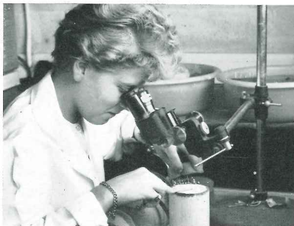
A SYRINGE ORDERLY EXAMINING THE POINT OF THE NEEDLE UNDER MICROSCOPE TO ENSURE THAT IT IS SHARP.
