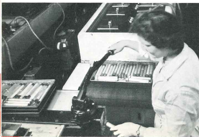
A SYRINGE ORDERLY SEALING THE LOADED CONTAINER WITH A FOIL CAP. A TRAY OF SEALED SYRINGES AND CONTAINERS ARE BEING STERILIZED BY PASSING THEM UNDER A SERIES OF HIGH TEMPERATURE 'INFRA-RED' HEATERS.
